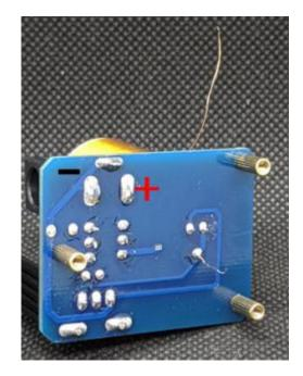
**9.** At this point the Kit is completed! Attach a DC power source between 9-12V to DC jack or to the Positive and negative rail of the board. This has been labeled in the photo above. The tesla coil can be tested using the included tester LED. When the power button is pushed, the blue led will illuminate the center of the coil and when the tester LED is brought near, the tester LED will turn on.
